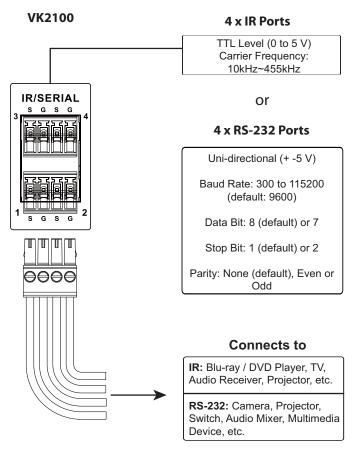
**IR Connection:** Connect a transmitter cable to the IR and Ground ports on the Control Box and install the IR transmitter on or near the device's IR receiving port, as shown on page 29.
