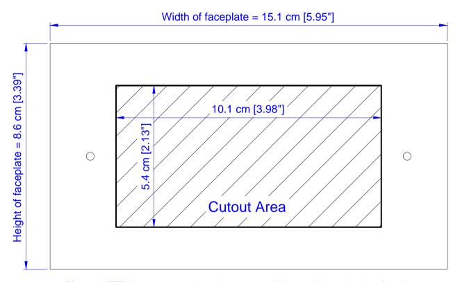
**Note:** ATEN recommends a 2-gang wall box with a depth of at least 6 cm (2.36 inches) to accommodate the connectors and cables.
